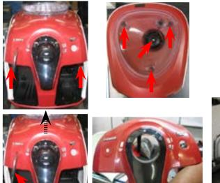
Remove the dreg drawer, water tank, mushroom finger protection device on the coffee container lid and coffee container, then loosen the screws shown.
