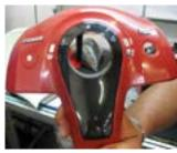
Slide out the steam hose protection, lift the cover at the rear by pressing down gently on the cooling vents to help detach the anchoring tabs, then pull it away from the steam hose, taking care not to scratch it.
