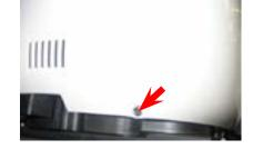
Loosen the screws shown and slide out the side cover; be careful of the protrusions (A) on the base.
